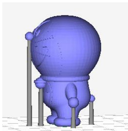
**Umbrella-shaped support :** ① top multi-point: Hold down “shift” to select the point where you want to add support (2 points or more), and finally release shift when you select the drop point.② point-to point: Hold down “shift” to select one point where you want to add support, and finally release the shift when you select the drop point. Set the support top and bottom radius and support height.
